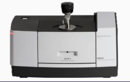
Portable gas chromatography mass spectroscopy (GC-MS)
